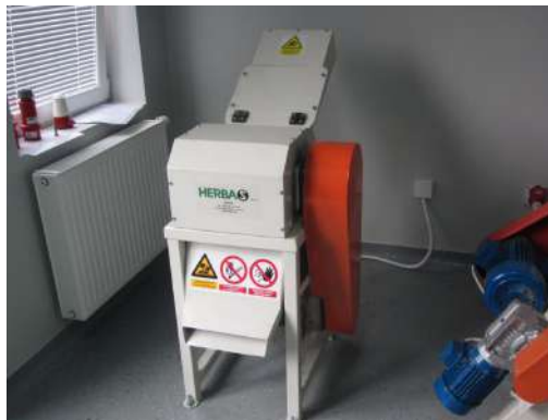
SMASHER OF PUMPKIN RESIDUE MASS AFTER MOLDING
