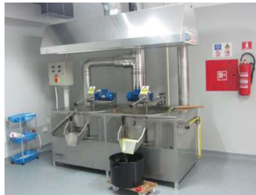
GAS STOVE FOR THERMAL TREATMENT OF THE MILLED MASS
